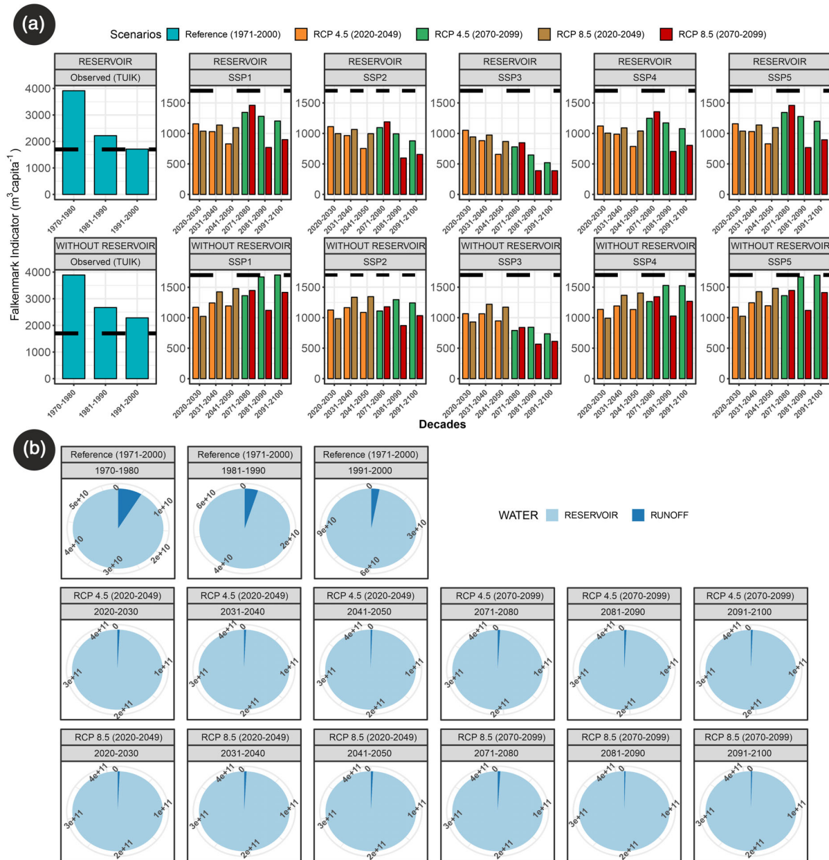
FIGURE 5 (a) Falkenmark indicator results based on climate and population scenarios (dashed lines indicate no scarcity or water stress), (b) ratio of water ( \text{m}^3 ) in runoff and reservoirs
