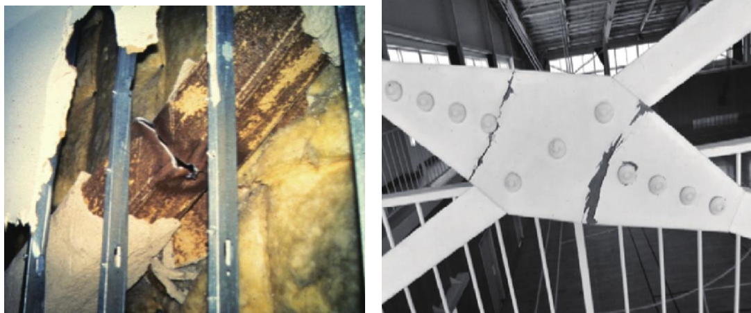
Figure 1.4. Brace fracture in CBFs (Engineering Mechanics, 2020, 37(10))
