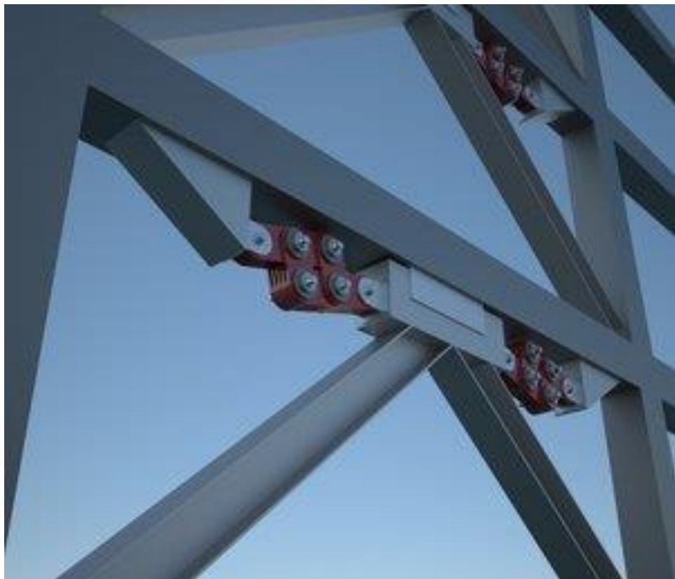
Figure 1.5. Braced frames with dampers. (Damptech company site)
