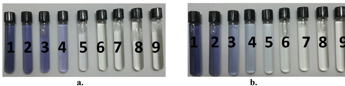
Figure 3. Color change during ozone treatment for a. 0.1 g/l dye solution b. dye and additives together (1- Control (Untreated dyestuff solution). 2- 2.5 min. ozone . 3- 5 min. ozone . 4- 7.5 min. ozone. 5-10 min. ozone . 6- 12.5 min. ozone. 7- 15 min. ozone. 8- 17.5 min. ozone 20s ozone 9- 20 min. ozone)
