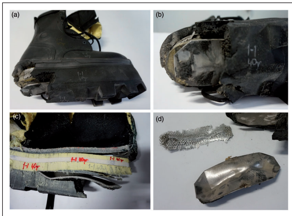
Figure 14. Damage pattern of sample Type-1 after the blast test: (a), (b) sole view; (c) cross-section view; and (d) deflector.
