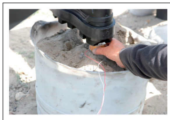
Figure 6. Explosive placement before the blast tests.
