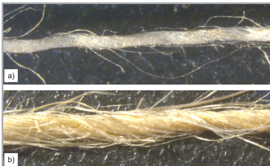
Figure 2. Surface images of flax (a) and jute (b) yarns used in the fabrics.
