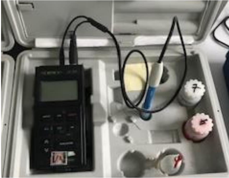
Şekil 3.5. WTW pH 330 model pH metre
