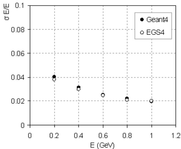
**Figure 3.** Energy resolution of the 3x3 crystal calorimeter for incident electrons of 0.2, 0.4, 0.6, 0.8, and 1.0 GeV.
