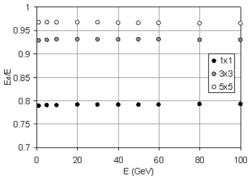
**Figure 5.** Deposited energy fraction as a function of incident electron energy.
