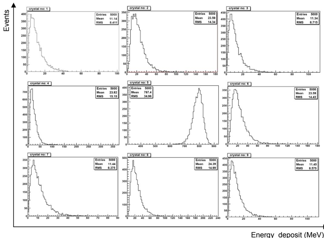
**Figure 1.** Energy deposits in 3x3  $\text{PbWO}_4$  crystals for 1 GeV electrons injected into the center of the central crystal.
