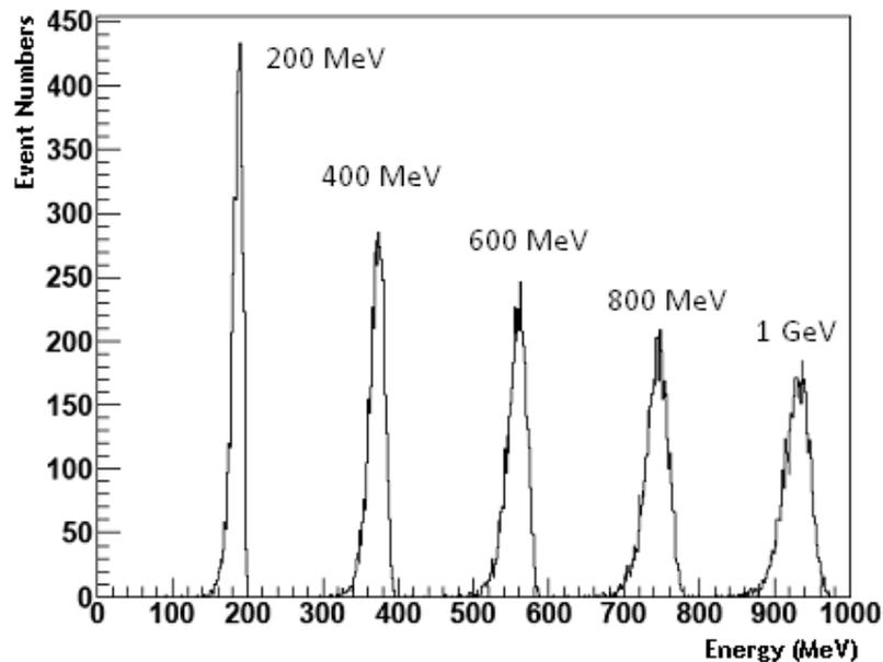
**Figure 2.** Energy spectra obtained by summing up all energy deposits in the nine crystals.
