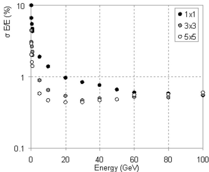
**Figure 6.** Intrinsic energy resolutions as a function of incident electron energies.
