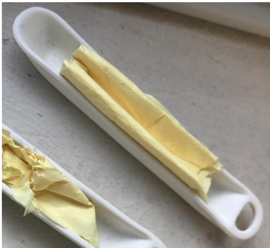
Figure 3.6. Prepared precursor PAN/Law nanofibers
