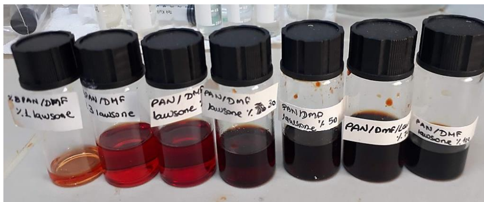
Figure 3.4. The prepared PAN/DMF/Law solutions
