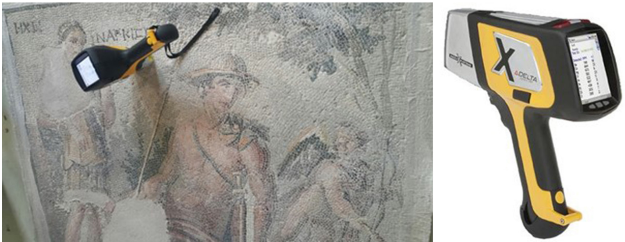
Figure 4 P-EDXRF spectrometer used in this study.
