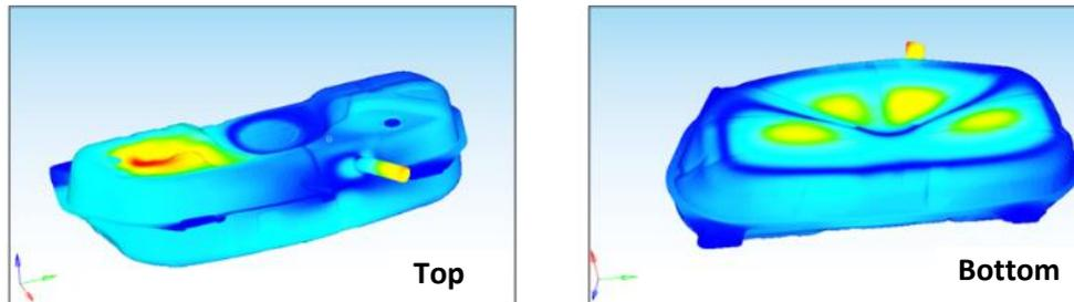
**Figure 14.** Two structural modes of the fuel tank (top and bottom) close to the rotational frequency of the FDM pump.
