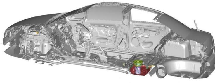
**Figure 16.** Location of a fuel tank on a passenger car
