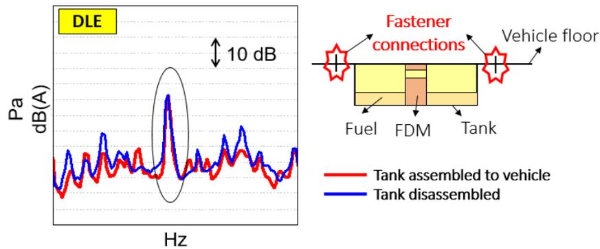
**Figure 18.** The effect of disassembling the fuel tank from the vehicle body
