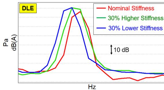
**Figure 10.** Effect of spring stiffness on the noise level at Driver Left Ear (DLE)
