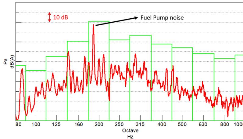
**Figure 3.** The frequency spectrum of noise measured by the microphone at the DLE.
