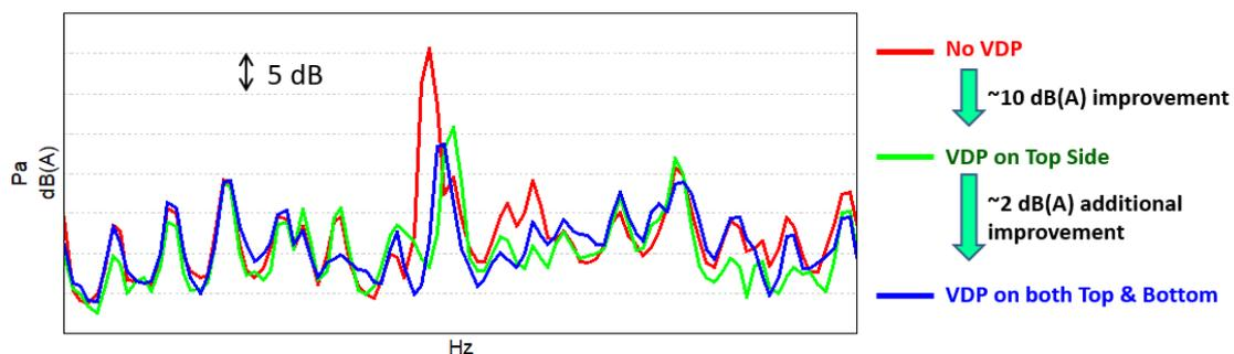
**Figure 15.** Improving effect of the VDP applications on the noise level (measured at DLE on the vehicle).
