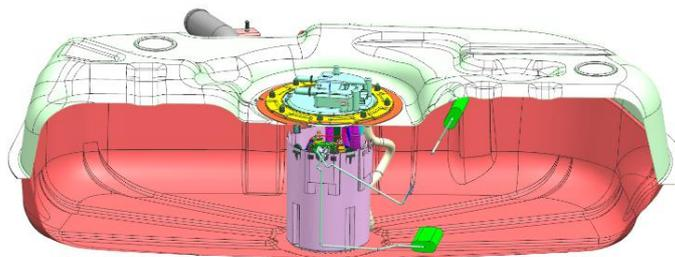
**Figure 2.** Fuel tank with fuel delivery pump mounted on it
