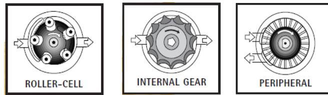
**Figure 1.** Three types of fuel pumps commonly used in the automotive industry
