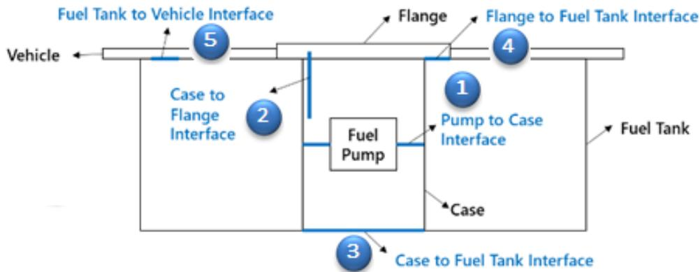
**Figure 5.** Schematic of the FDM-Fuel Tank-Vehicle Group
