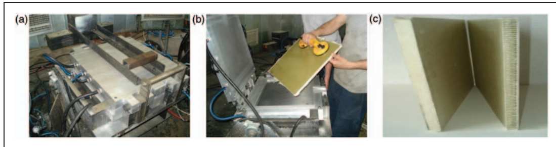
Figure 3. Fabrication steps of foam filling process (a and b) and view of foamed and unfoamed panels (c).
