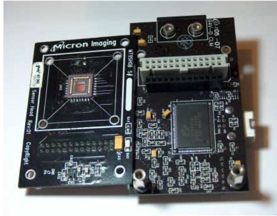
Figure 9. Micron DAQ setup: the MT9V011 sensor with its DAQ board (Demo2).
