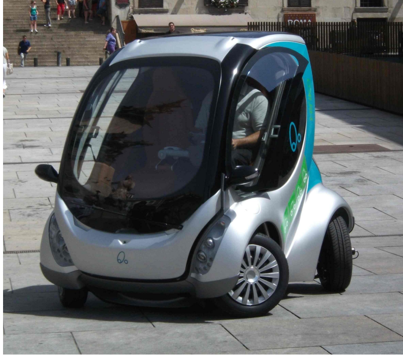
Figure 2.20. Hiriko fold — a vehicle employing in-wheel motors
