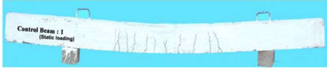
e) Experimental Crack Pattern at Failure Load (49.5 KN)
