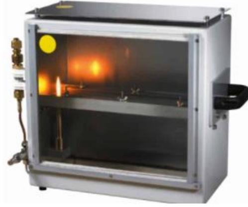
Şekil 3.19. Yanma kabini ( https://info-tek.com.tr/fmvss-302-fmvss-302-iso-3795-astm-d5132-04 )
