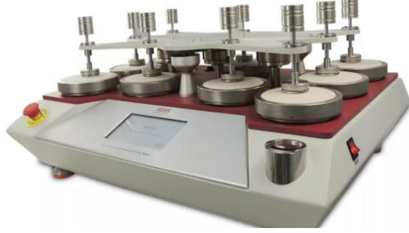
Şekil 3.18. Martindale aşınma test cihazı ( https://www.testertextile.com/product/martindale-abrasion-pilling-tester-tf210/ )
