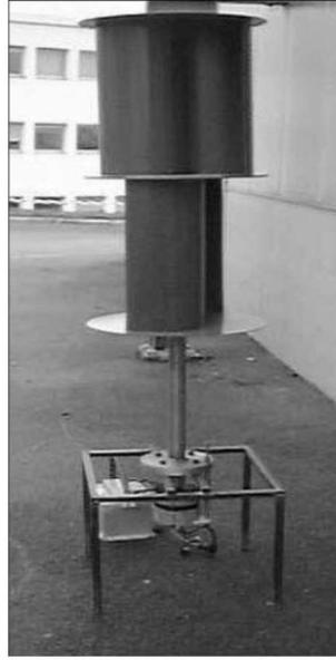
**Şekil 2.3.** Savonius Rüzgar Türbini Prototipi (Menet, 2004)
