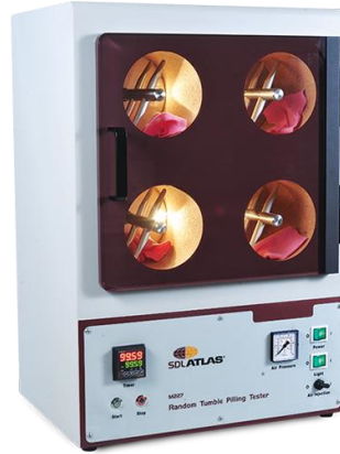
Şekil 3.5. SDL Atlas düşey taklalı boncuklanma test cihazı ( https://sdlatlas.com/products/random-tumble-pilling-tester )
