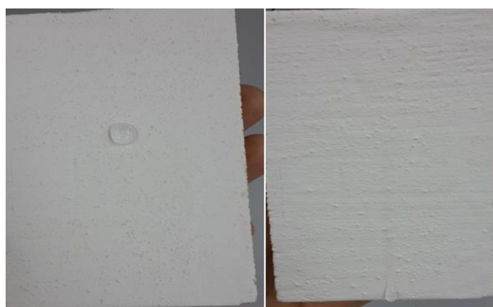
Figure 7: Hydrophobicity test result for No:3
