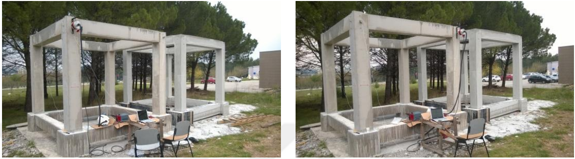
Figure 3.7. The working space of two frames when waiting for the age of concrete.
